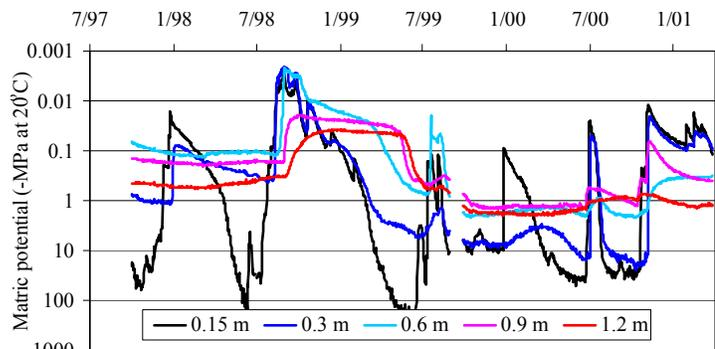
Figure 3. Matric potential in the GCL/asphalt barrier
